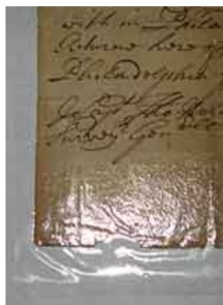
Figure 5. The wrinkling of this laminate may place great stresses on the paper enclosed within it. This image also shows the high surface gloss and surface texture that may be present on laminated papers. 18th century land grant from the Pennsylvania State Archives
